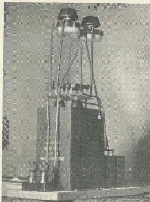
Another view of the resistance chain. The controls are mounted on the top panel of the framework.
